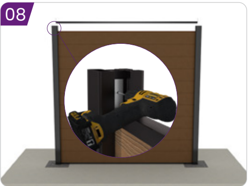
08 Fix L-clips to the post with self-drilling screws.
