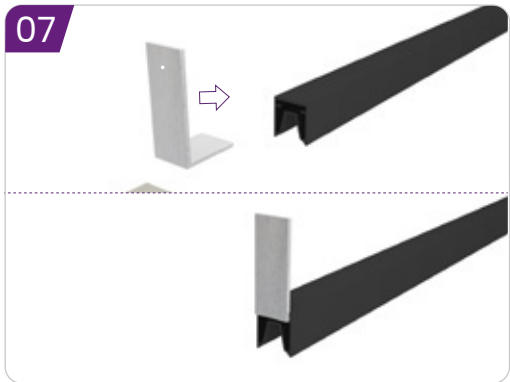
07 Attach L-clips to each end of the top fence board and put them into position.
