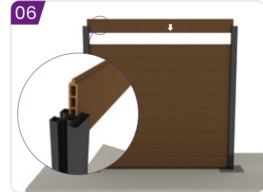
06 Slide the next fence board onto the post, ensuring it is straight. Continue installing fence boards.
